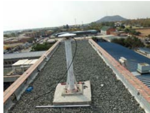
Figure 2: An installed Trimble NetR9 GNSS Receiver
